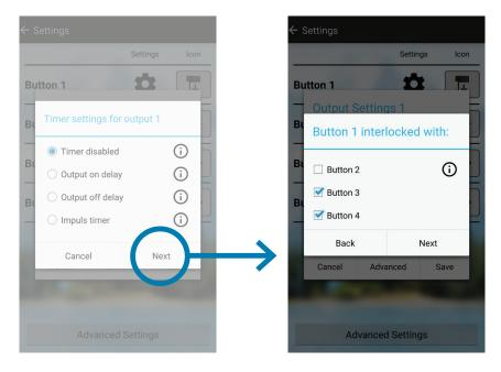
Setting an interlock between two or more buttons will prevent the outputs from being active at the same time.
