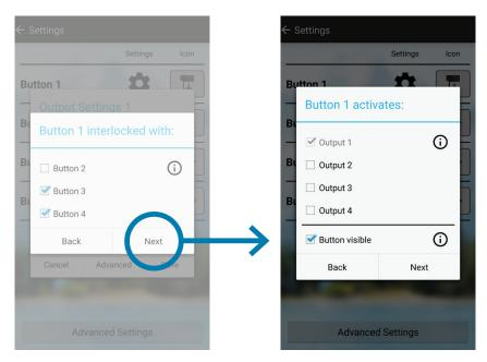
The selected outputs are activated if button is pressed.
